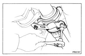
2. REMOVE CENTER SUPPORT BEARING FROM BODY
