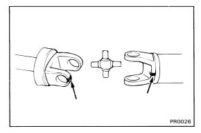
(b) Align the matchmarks on the yoke and shaft.
