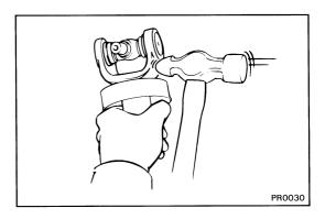
(b) Using a hammer, tap the yoke until there is no clearance between the bearing outer race and snap ring.
