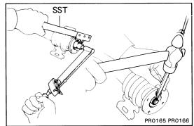
(c) Using SST to hold the flange, press the bearing into position by tightening down a new nut.
