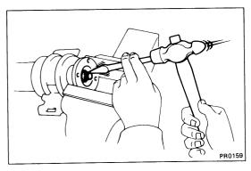
2. REMOVE CENTER SUPPORT BEARING FROM INTER-MEDIATE SHAFT
