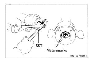
(b) Using SST to hold the flange, remove the nut.
